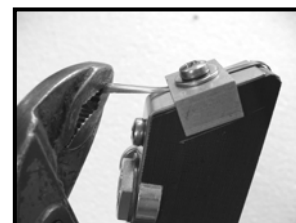
Pull the wire tight in second clamp plate using a pair of pliers and a vice.
