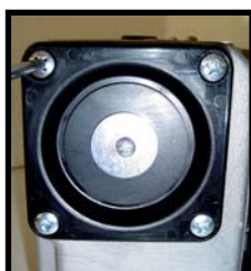
Unscrew the cover from the filter housing
