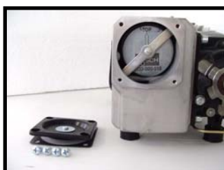
The filter(s) is/are visible behind a tensioner
