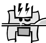
1-2 CUT-OFF SEAL 1 x 3,5 mm seal 1 x 1,1 mm cut individual time
